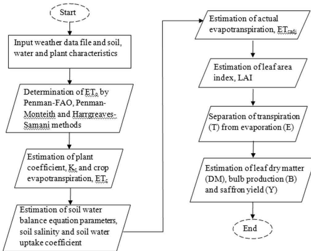
Figure 1. The flow chart of the modified Saffron Yield Estimation Model.
